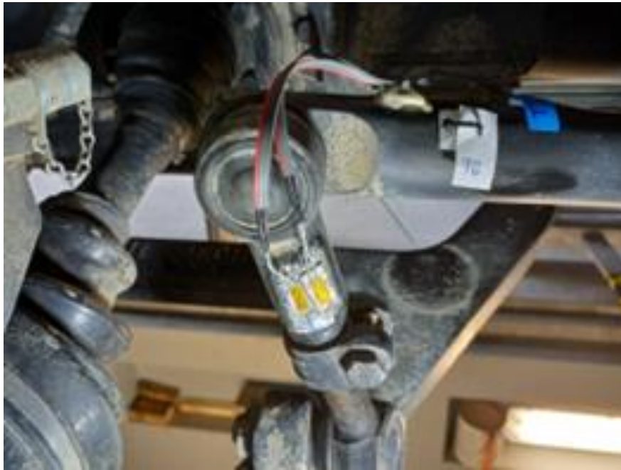
Fig. 3 Measuring the tension in the wheel suspension
