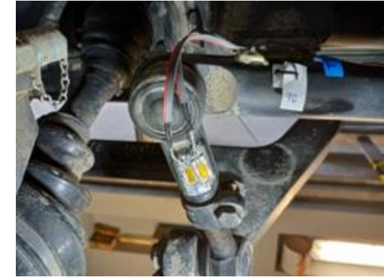
An example of tensiometric measurement of the mechanical stress of the structure of special vehicle
