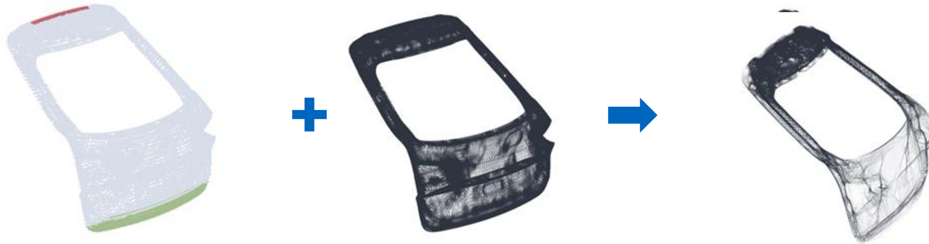
Fig. 5 Strength calculation model of the rear door of a passenger car
