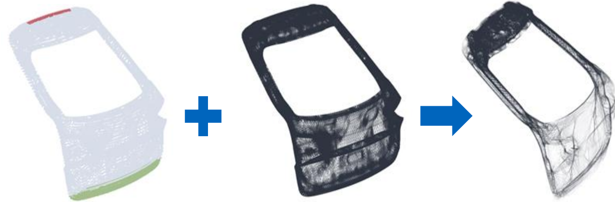
Strength calculation model of the strength of the rear door of a passenger car
