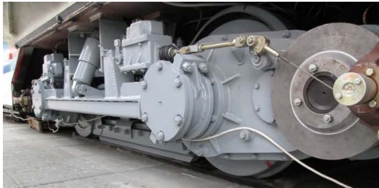
Typical design of a split brake on a low-floor tram
