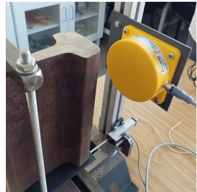
A test fixture for a basic test of its sensor sensitivity
