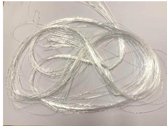
Glass fibers in the form of roving - R-310 – S-2 Glass
