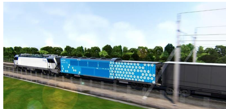
Hydrogen energy tender concept for electric locomotives
