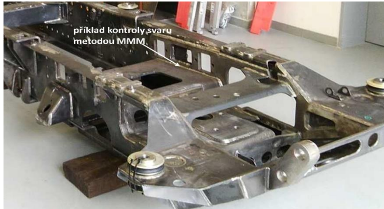
Inspection of the welded frame of a special vehicle by the method MMM
