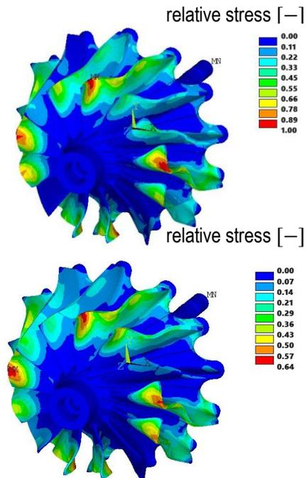
The vane modification produced a reduction of blade max. stresses by 36 %.
