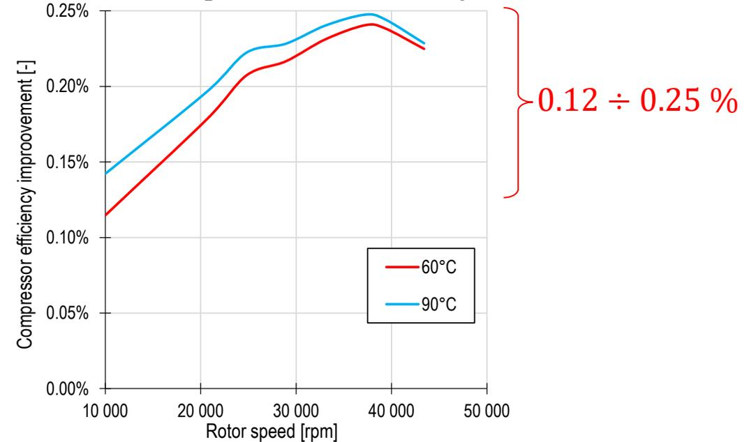
Decreasing the disc friction on the compressor wheel has only **small effects** on efficiency under **high-speed** conditions. The effects under low speeds are mostly insignificant.
