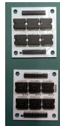
RICE GaN inverter 10kW@1MHz for auxiliary PSU
