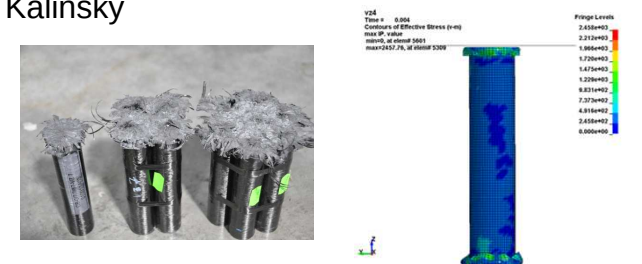
Experiment – composite tubes
