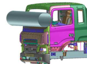
Cab test acc. to ECE R29 incl. validation test
