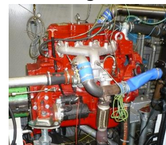
Gas diesel(dual fuel) engine - vehicle turbocharged diesel engine CUMMINS ISBE-150 (EURO 4 - 4BTA)
