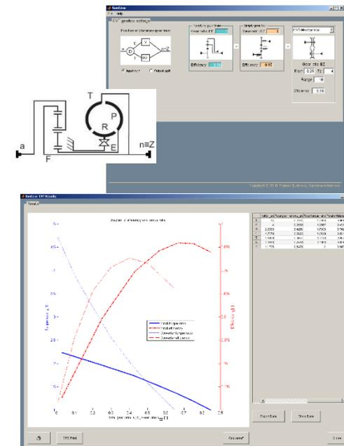
Program for complete analysis of morestep planetary gearboxes consisting of maximally 4 single planetary sets of arbitrary type.
