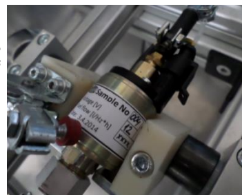
Prototype of fuel pump, burner and combustion chamber
