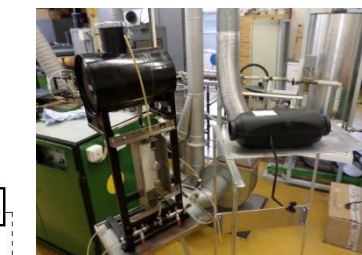
Test bed BRANO burner and combustion chamber experiment
